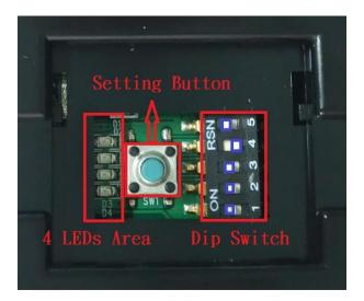
C) Turn on the power, then LED will flashing. When LED is flashing, then turn off the power.
