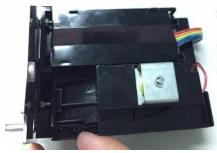
1. 先扳開下方卡榫 1. First, disassemble the lower mounting clip.
