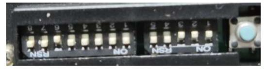
The 6ty inhibited transaction mode : Non-Inhibited transaction ( turn Dip Switch no. 6,8 to up ; no. 7 to down )
