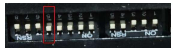
Pulse output for Normal Low ( turn dip switch no.5 to down )  $% \left( {\left[ {{{\rm{Normal}}} \right]_{\rm{Normal}}} \right)$
