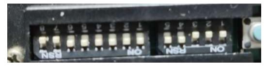
The  $5^{th}$  inhibited transaction mode : depending on inhibit signal ( turn Dip Switch no. 6 to up ; no. 7, 8 to down )
