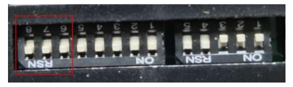
The  $1^{st}$  inhibited transaction mode ( Select inhibited transaction mode ) ( turn dip switch no. 6,7,8 to all down )
