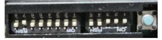
The 4th inhibited transaction mode ( Select inhibited transaction mode ) ( turn dip switch no. 6 to down ; no. 7, 8 to up )
