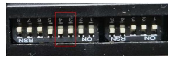
The  $\mathbf{1}^{\scriptscriptstyle{\mathrm{st}}}$  pulse width ( turn Dip Switch no. 3 , to down )
