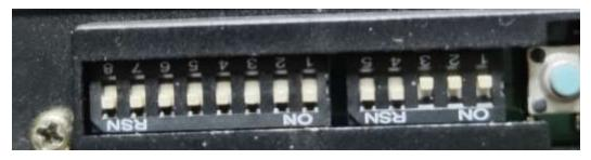
The 2nd inhibited transaction mode (Select inhibited transaction mode) (turn dip switch no. 6,7 to down, no. 8 to up)
