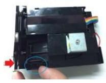
3.從新頭所指的方 向屬用力推入,將 其(藍圈)卡榫扣上 3. Push the plate (red arrow) hard so as to assemble it.
