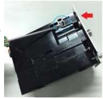
2.從解頭所指的方像處推 人·將莫(藍團)卡榫扣上 2. Push the plate ( red arrow) hard so as to assemble it.
