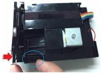
3.從箭頭所指的方 向處用力推入,將 其(藍圈)卡榫扣上 3. Push the plate (red arrow) hard so as to assemble it.
